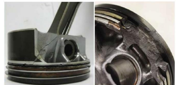
Two examples of piston damage due to LSPI observed during testing at Southwest Research Institute ® http://www.infineuminsight.com/insight/may-2015/investigating-low-speed-pre-ignition
